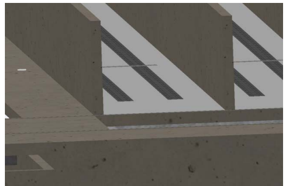
Photo 7 - Baseplate embedded in the tunnel floor
