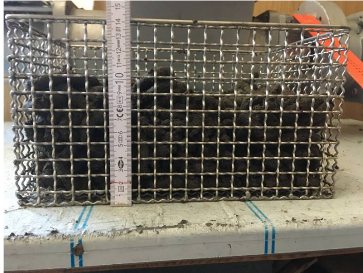
Figure 8: Height of the sludge before drying process - 10 cm in average
