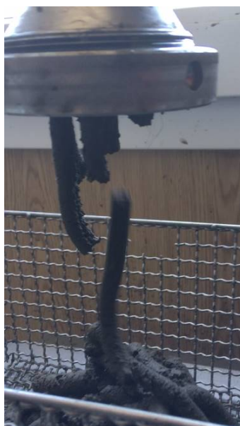
Figure 6: Extruding process, max. pressure: 1.0 bar
