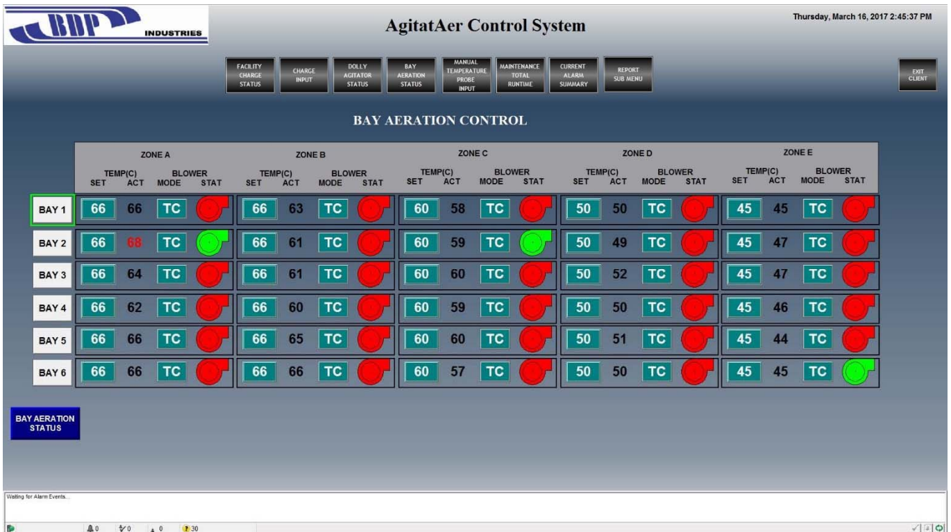
Photo 13 – Sample Blower Control Screen
