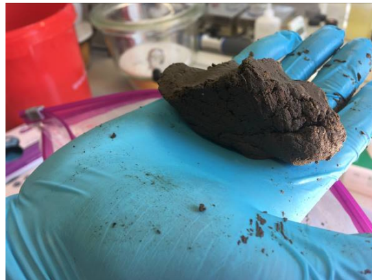
Figure 4: Formed wastewater sludge after arrival
